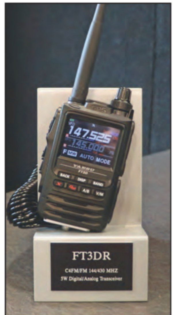
The new Yaesu FT3DR handheld offers 5 watts of analog FM or digital C4FM audio on 2 meters and 70 centimeters.
