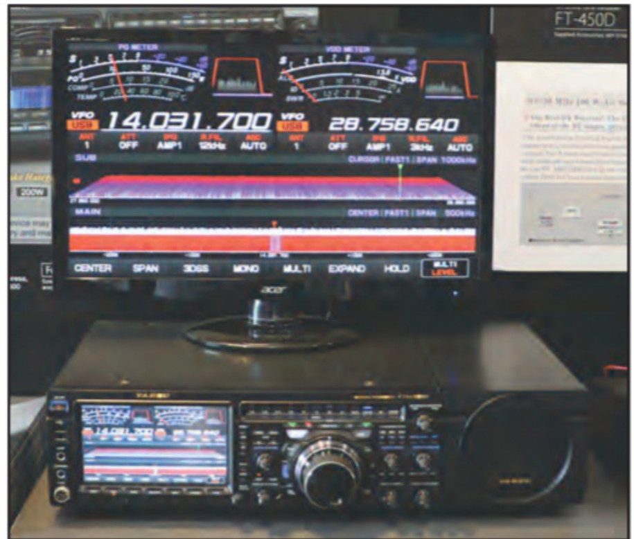
Named with a nod to the legendary FT-101 transceiver of the 1970s, Yaesu's new FTDX101D transceiver is a top-of-the-line software defined radio covering the HF bands plus 6 meters.
