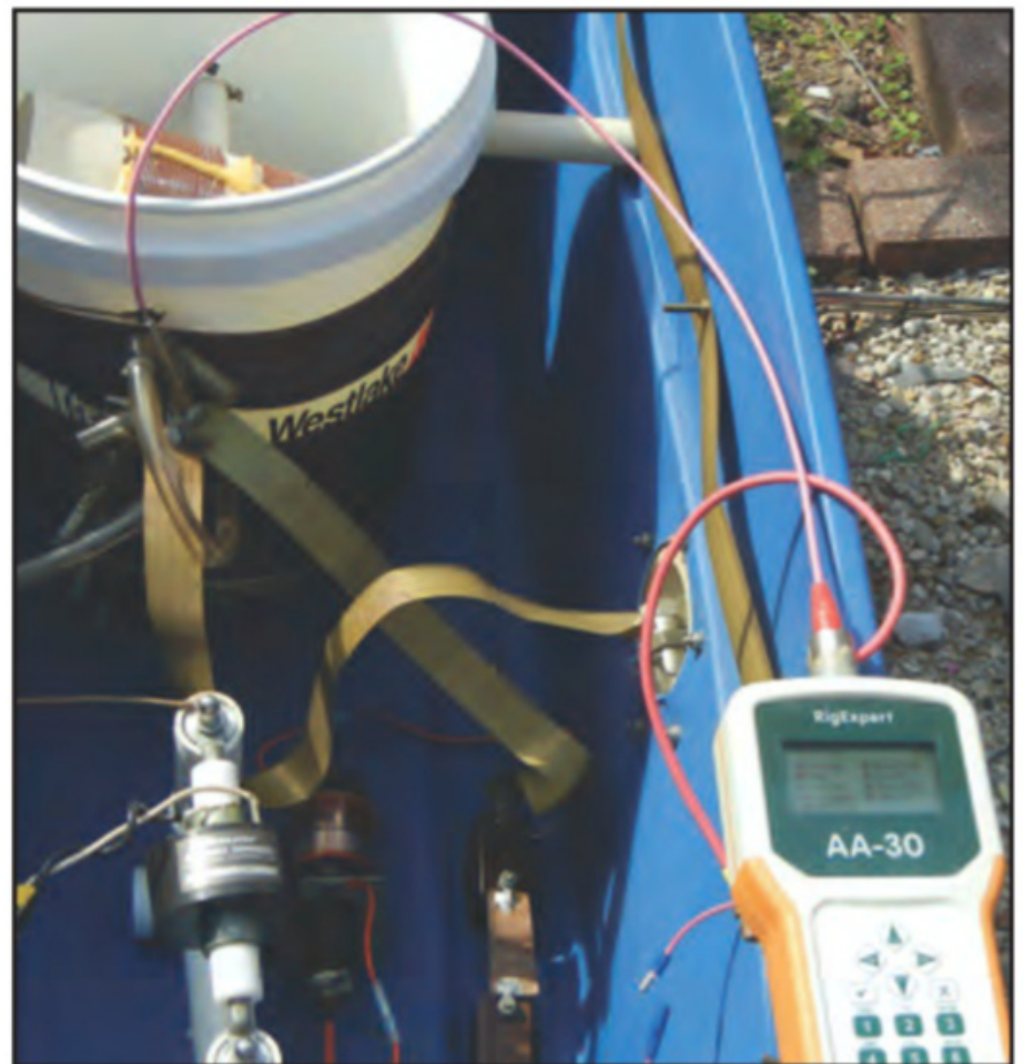
Photo B. This very busy image shows the common arrangement used at KB5NJD for measuring total system resistance. The center conductor of the analyzer (pink wire) interfaces with the input of the loading coil. The ground lead (red wire) connects to the ground bus in the antenna-tuning unit (ATU). Note that the ATU ground jumper can be seen disconnected in the lower right of the image. This removes the LC matching network from the circuit for the purpose of these measurements. The coax is also disconnected at the input of the ATU (not shown).
