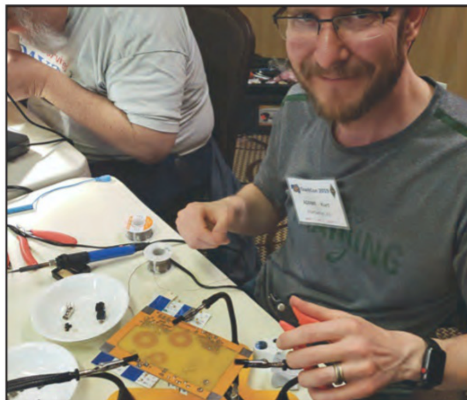
Kurt Zoglmann, ADØWE, uses a rather unique board holder made from stiff wires and alligator clips.
