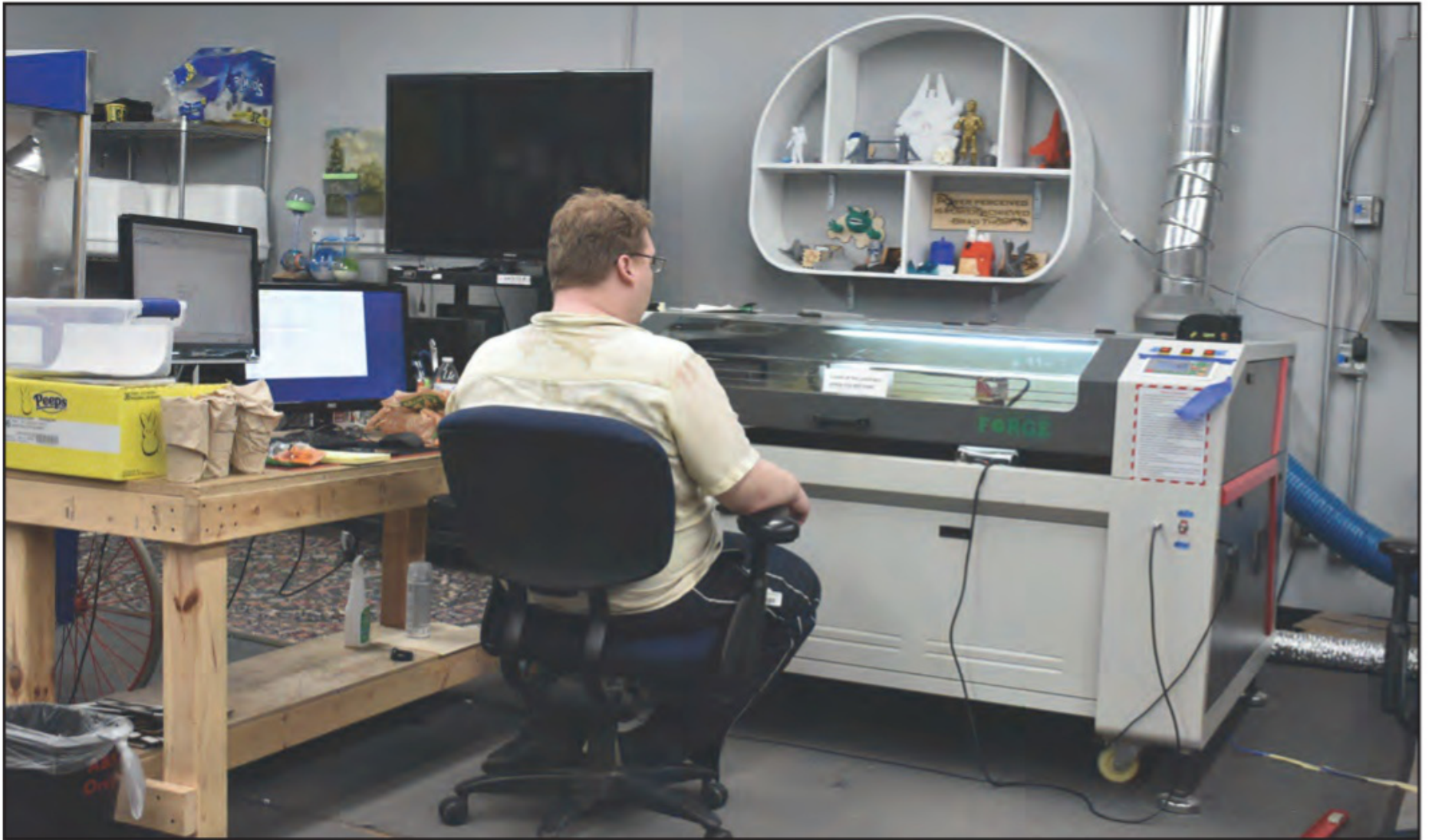
Photo H. IFMS 100-watt laser available to members.
