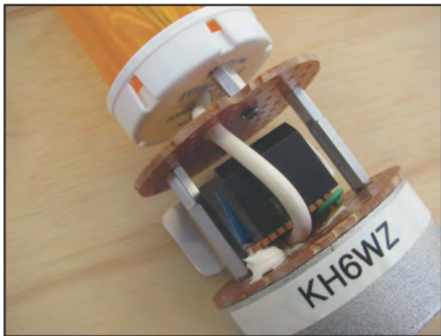
Photo B. This is a view of the high-voltage circuit for the miniature Tesla coil for Maker Faire and similar educational demonstrations and events.
