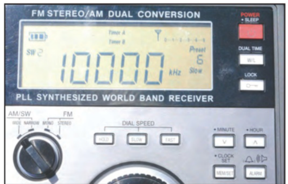
Photo D. A portable shortwave set can help track grow-light ballasts.
