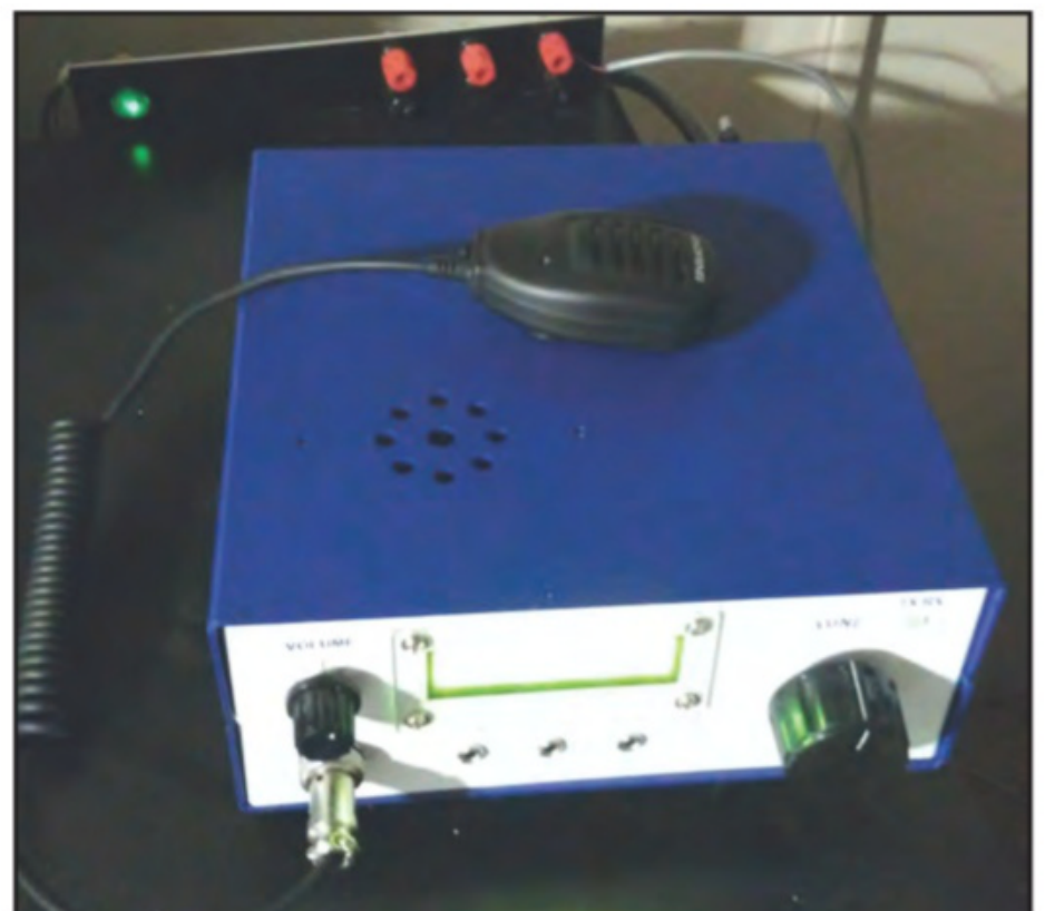
Photo G. Completed project powering a µBitx transceiver.
