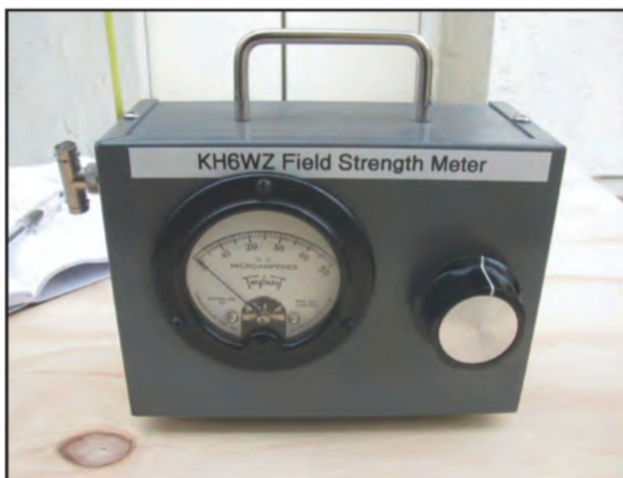
Photo C. I always wanted to build a field-strength meter, and finally completed one. It is a simple and useful piece of test equipment — and an excellent item to demonstrate radio frequency energy at Maker Faire events.
