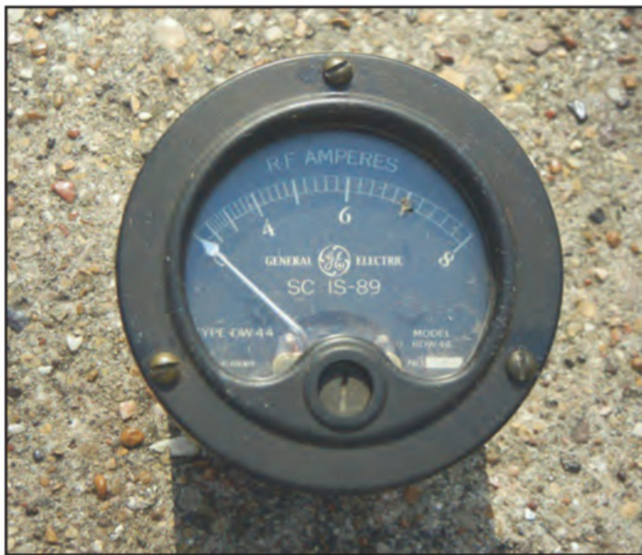
Photo A. Here is a common General Electric thermocouple-type RF ammeter. For vertical antennas, the meter leads can be inserted in the output lead of the antenna tuning unit to the antenna, but mount the meter as if it were at high potential to avoid arcing to other objects and creating bigger problems. With loops, simply insert the meter anywhere in the loop circuit. Near the feedpoint is often the most convenient location, but for small loops, current distribution is relatively constant so it can be inserted anywhere along the radiator.
